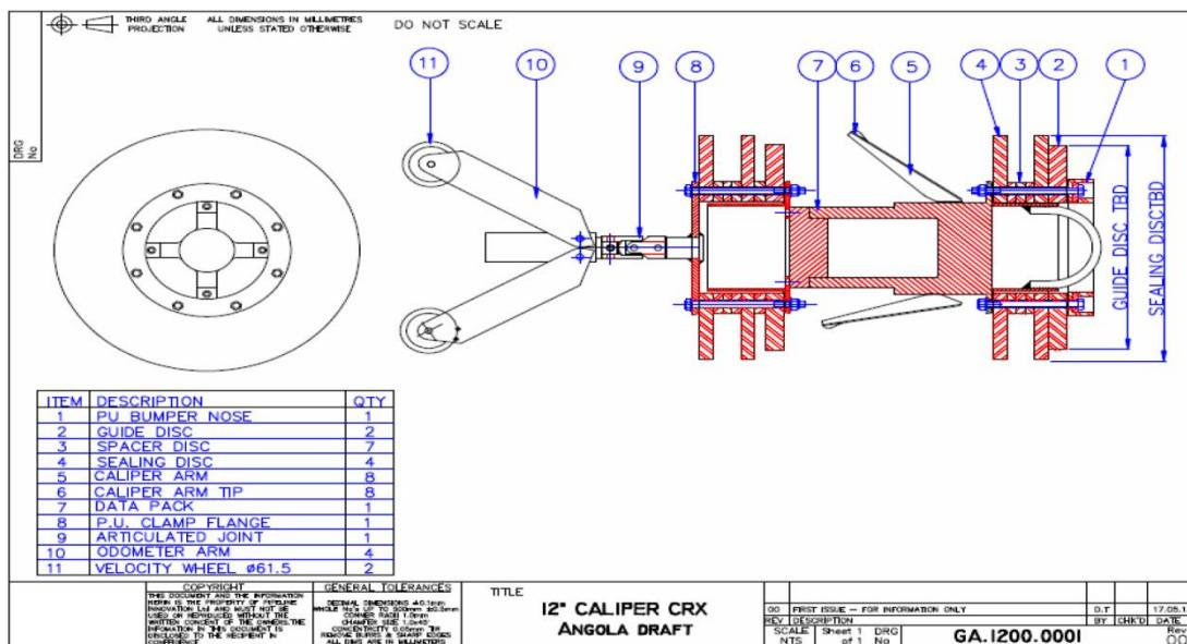
Figure 5—Segment W 12-in. caliper pig
