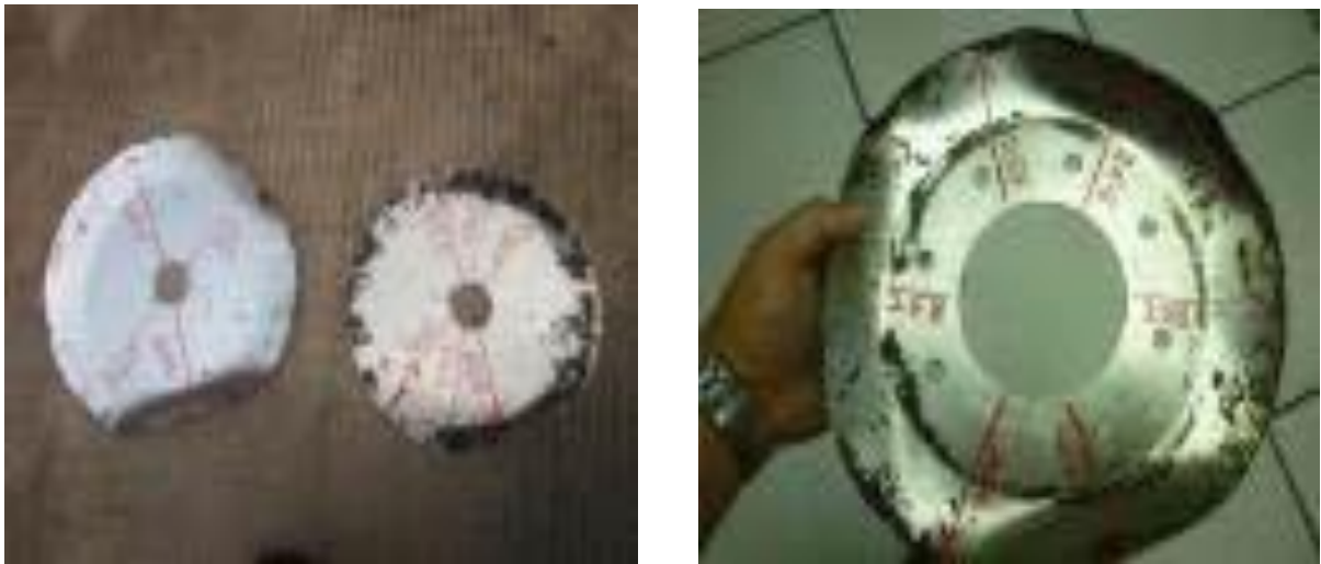
Figure 1: Examples of damaged gauge plates
