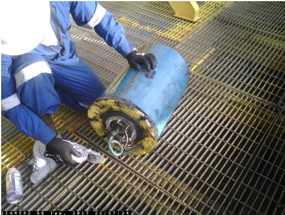
Figure 1: SmartFoam™ tool equipped with rear mounted DDMD at receive
