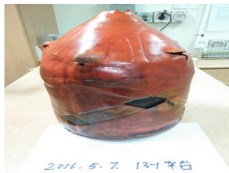
Figure 2: Operator’s pig at receive
