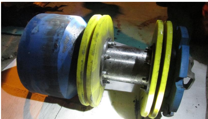
Figure 3: Pioneer™ tool at receive onshore in good condition
