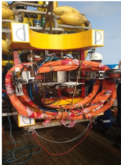
Figure 4: MEC-Hug inspection tool and Work Class ROV before dive
