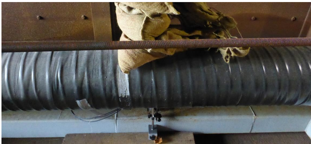
Figure 7 6kg sandbags applied to the centre of a 3m length of MASiP pipe
