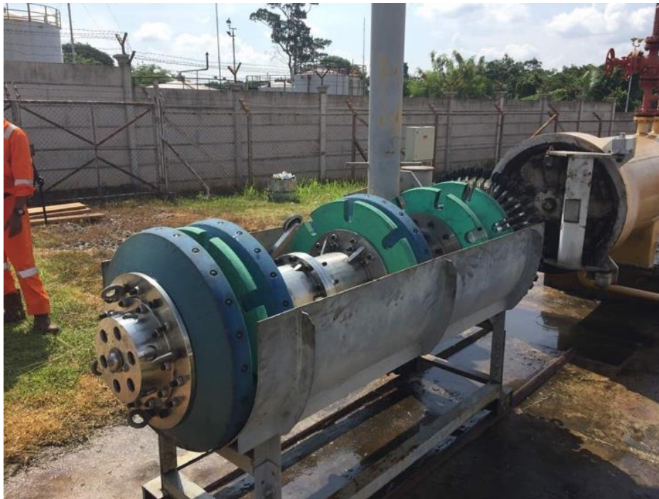
Figure 3: Receiving the 28" High Resolution Geometry + IMU Survey Tool
