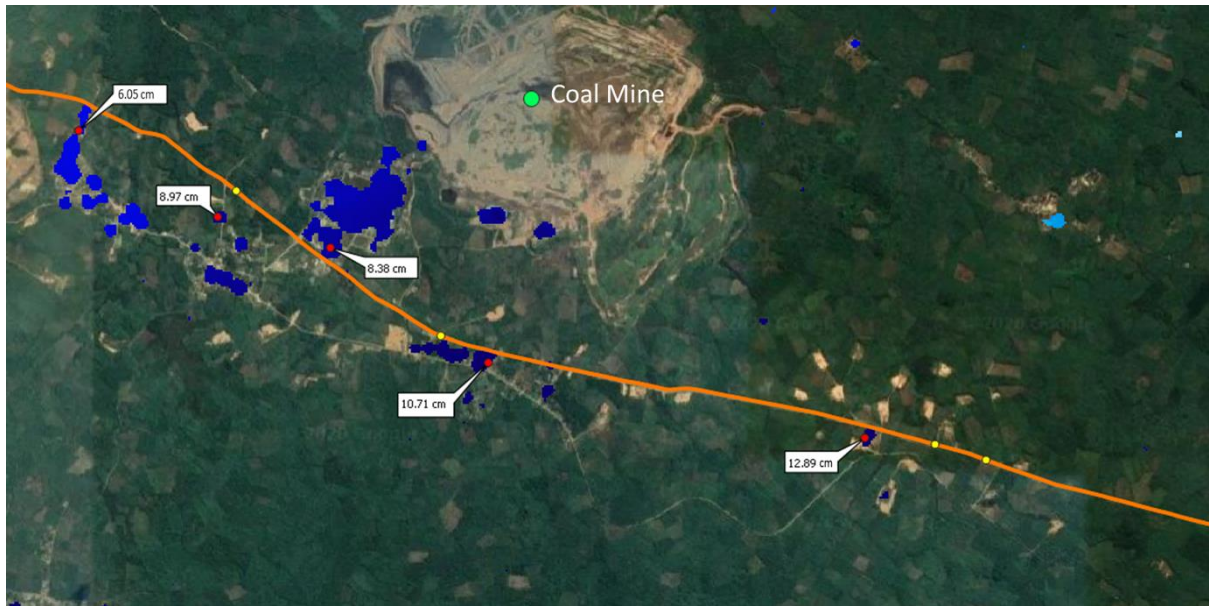
Figure 6: SAR Pipeline Image of 4 high strain points near the coal mine and one near the river
