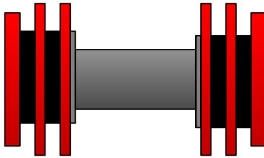
The various elements of the pig are attached, using multiple bolts, to a solid body or mandrel.
