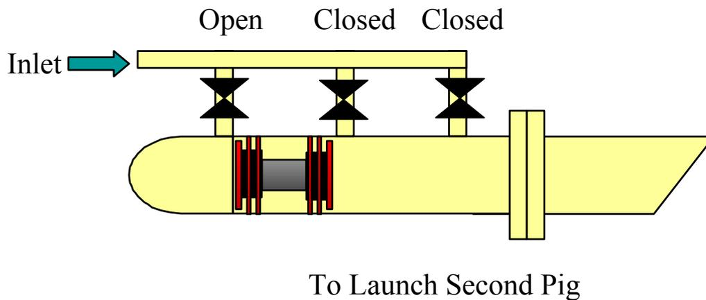
The pig trap can also feature additional ports for pressure/temperature monitoring, chemical injection, pig signalling, etc.
