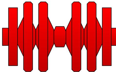
Both sealing and guide elements are cast as a single component in polyurethane.
