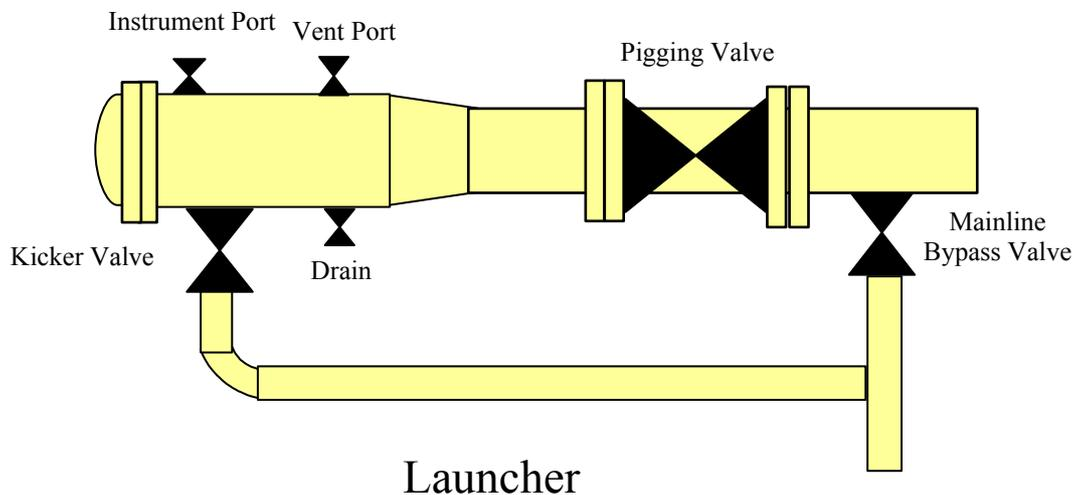
Again the same pig train can be launched from a multiple-pig pig trap by redirecting flow through pipework to allow individual pig launching as in the sketch below.
