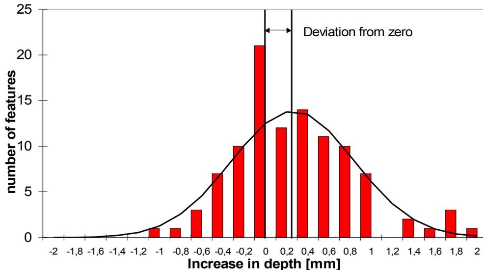
**Figure 2: The increase in depth for 104 sample pairs of metal loss features as a histogram. There is a deviation of the mean from zero, that cannot be explained by the pig measurement uncertainty alone.**
