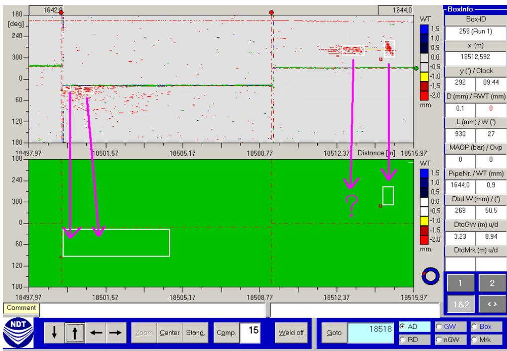
**Figure 1: A sample screenshot of the RunComparison Function of NDT's analysis Software. The purple (dark grey) arrows indicate what correspondences can be found.**
