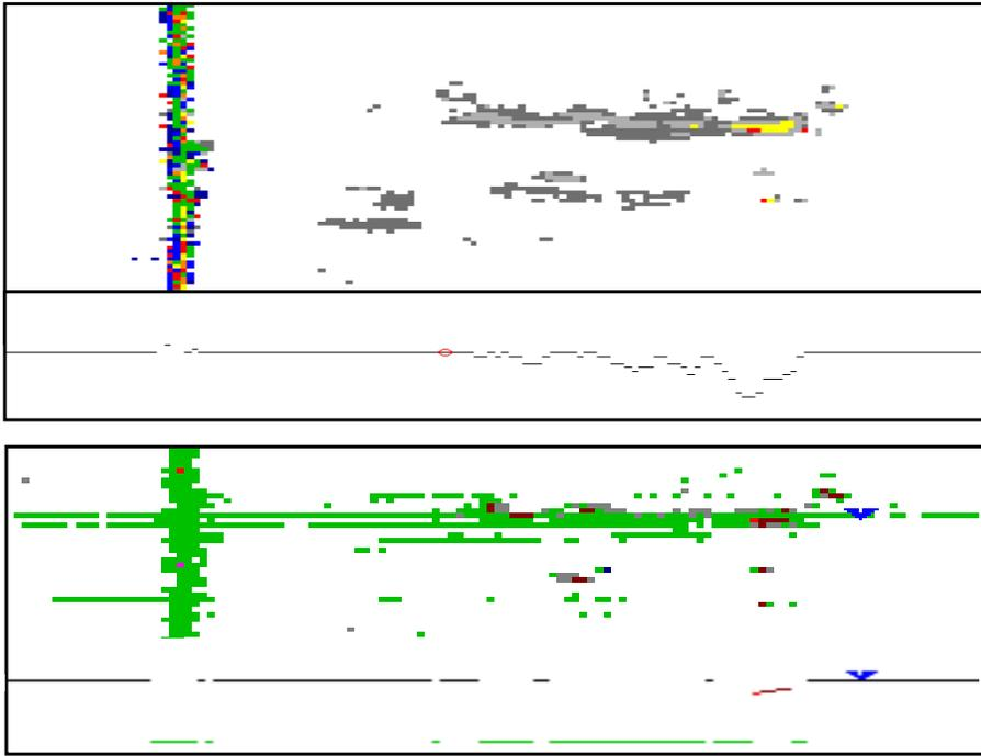
**Figure 3 A defect seen by two inspections with different UT-tools. The lower inspection is over 12 years old. The upper picture show the defect as it was seen recently by an NDT pig.**
