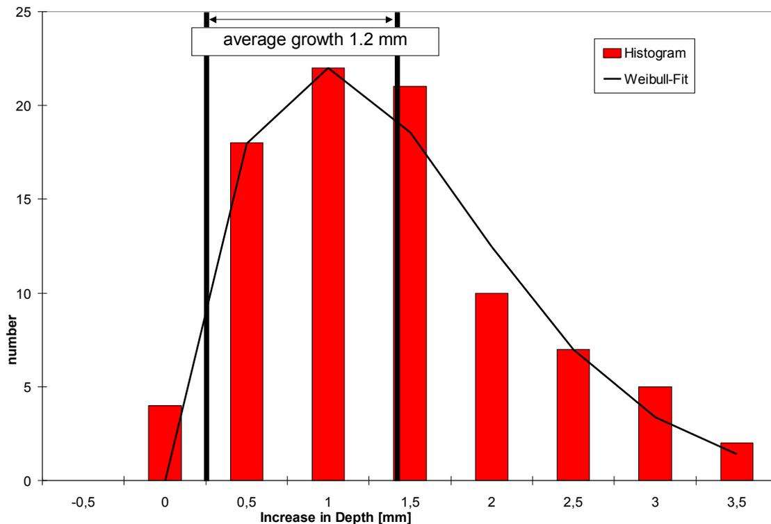
**Figure 2: The increase in depth for 89 sample pairs of metal loss features as a histogram. There is a deviation of the mean from zero, that cannot be explained by the pig measurement uncertainty alone.**
