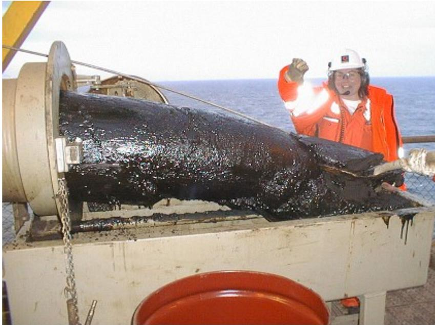
Figure 1 Part of a wax plug retrieved from the pig trap at Statfjord B after pigging the pipeline from Snorre B to Statfjord B (Sept. 2001)
