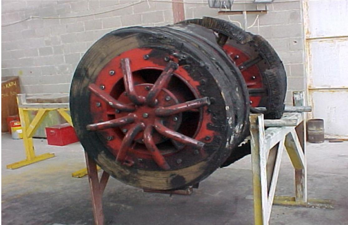
Figure 1: Cleaning tool after a 50-km inspection through black powder.
