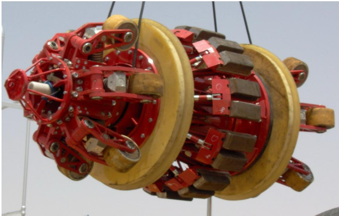
Figure 2: ROSEN 48" Black Powder Cleaning Tool before launching
