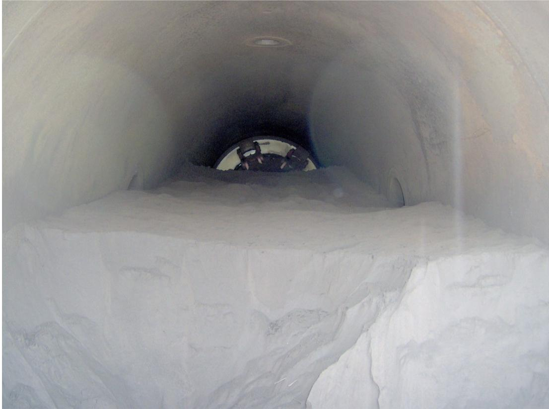
Figure 3: Receiver filled with black powder
