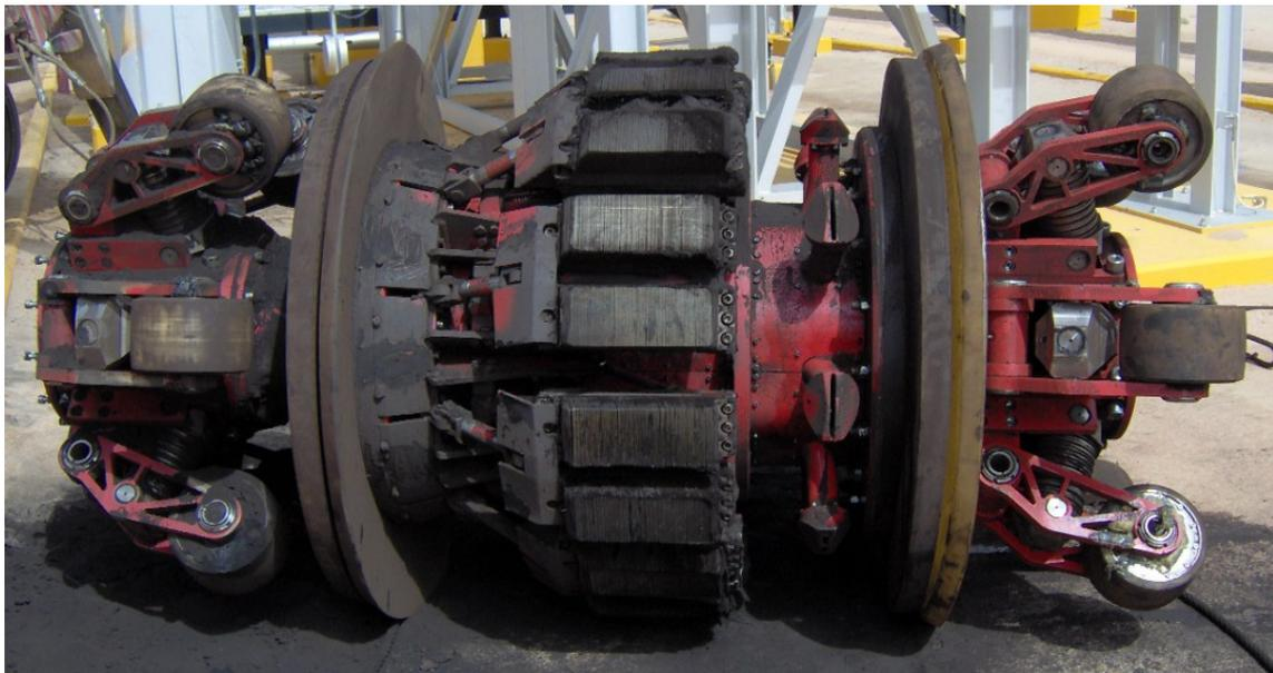
Figure 4: Cleaning tool after more than 170 km in a gas line containing dry black powder
